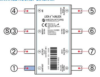
Each ADVANTAGE Hookup is comprised of multiple ports and connector assemblies. Each port is labeled with a Port ID number (circled). This same number also identifies the corresponding Connector Assembly.
