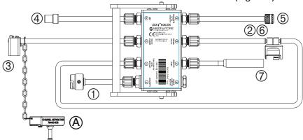
Each ADVANTAGE Hookup is comprised of multiple ports and connector assemblies. Each port is labeled with a Port ID number (circled). This same number also identifies the corresponding Connector Assembly. Each Connector Assembly is fitted with a specific endoscope connector. (see Fig. 2).
